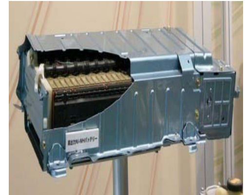
High power Ni-MH Battery from Toyota Prius
